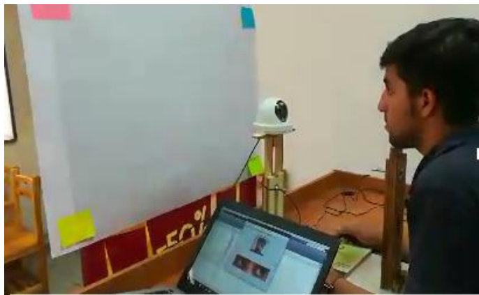
Figure 9. Experimental setup with four command point (corners) and one confirmation command (center)
